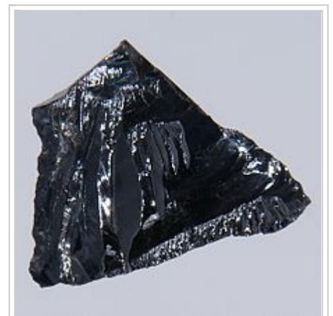
Silicon crystals are the most common semiconducting materials used in microelectronics and photovoltaics.
